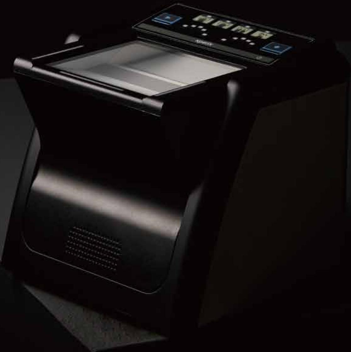
RealScan-G10 is a compact live-scanner for single and ten-print capture. Xperix's advanced optical technology allows high-speed image capturing and seamless image processing. IP65-rated dust and water resistant housing makes it suitable for indoor and mobile environments. With its proven reliability of FBI certification, RealScan-G10 is the perfect portable live-scanner for civil and criminal applications.
