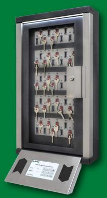
The keys are attached to intelligent keyfobs that have a built-in chip with a unique identifier and a three-millimeter stainless steel shackle. The data from the built-in chip is used to verify and identify the key every time you need to remove the key from the storage or put it back to its place. Only authorized users, whose rights are assigned individually, can have the access to a key. Keyfobs of different colors are available for order.
